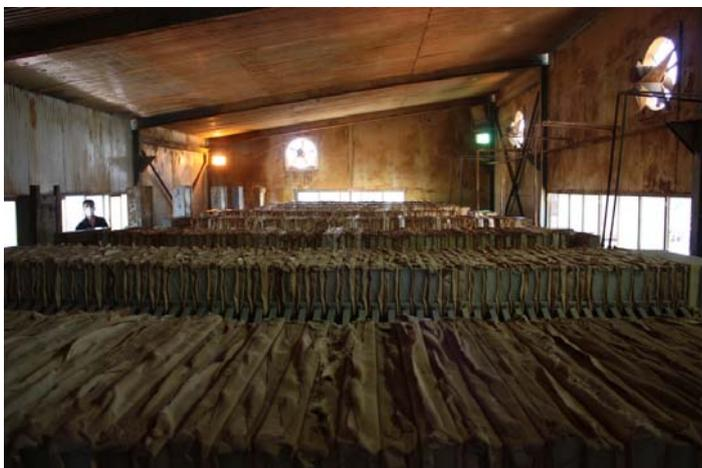
**A bank of filter presses, part of the existing zinc/lead ore processing operation that produces as a residue the 20% Zn+Pb feedstock to be recovered in the IRC Project**
