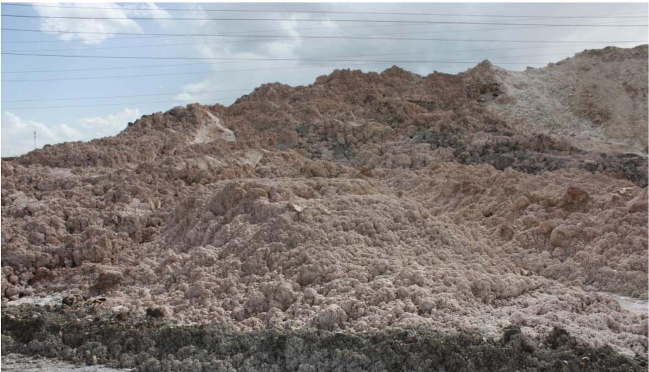
**A view of part of the very large stockpile of ~20% Zn+Pb residue feedstock for the IRC Project**
